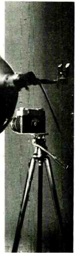
Fig. 3—Pin or tape the drawing to a suitable background such as a sheet or a white wall. (Second light is out of sight at right.)
