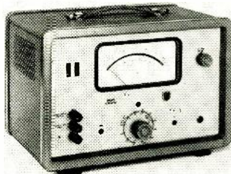
Philips GM 6020 micro-voltmeter. It indicates the polarity of the measured voltage automatically by lighting one of the two neon lamps marked + and -, at left.
