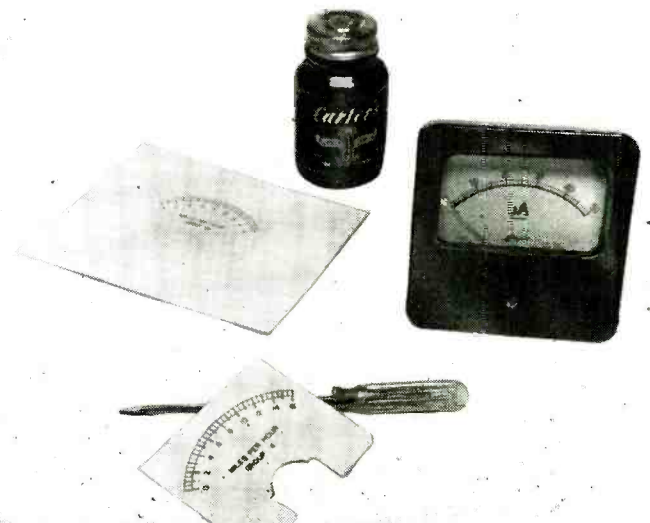
Fig. 6—Trim the print and glue it to the rear of the old meter scale.
