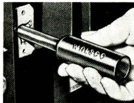
Fig. 5—Technician inserting high-voltage cheater into high-voltage interlock.
