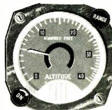
Fig. 10—Indicator of airborne FM radar used as altimeter.
